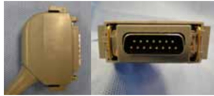
24. Rectangle, 15 Pins, Male, Locking Mechanism
